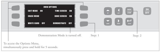
FIGURE 13: Enabling/Disabling the Demonstration Mode
